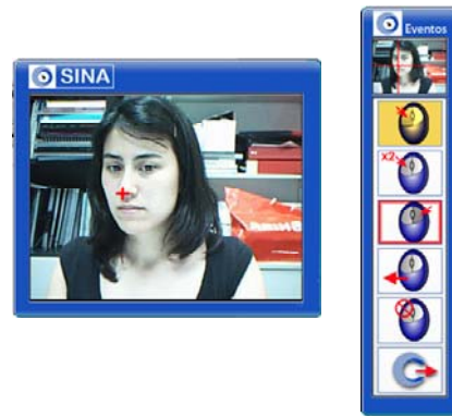
Fig. 2. Hands-free interface. Through head movements, the user chooses one option (left mouse button, double click, right mouse button, etc. similar events as a mouse).
