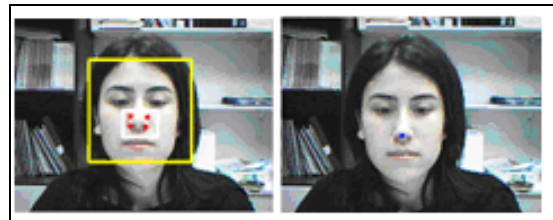
Fig. 4. (left) Best feature selection using symmetrical constraints; (right) Mean of all features: nose point.
